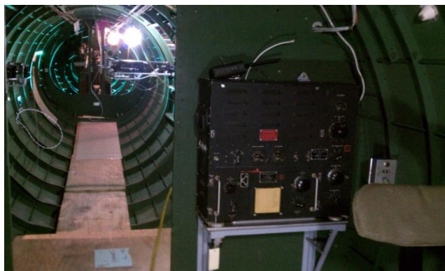
Newly installed BC-375 Liaison Transmitter
